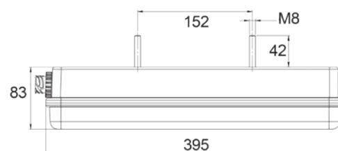
AMP socket placed on the side
